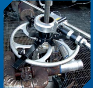
RS-2 operating a non-rising stem valve.
