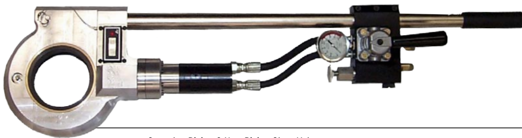
Operates Rising & Non-Rising Stem Valves
